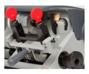
Two/three sided revolving clamps on the right for Abus® and Abloy® type keys
