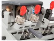
Four-sided revolving clamps on the left side for edge cut style
