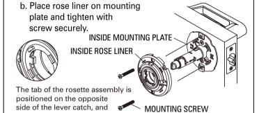
Use lever catch to press down catch in the hole and push inside lever all the way in until clicks into catch hole.
